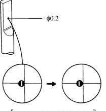
Aperture  $\phi$ 0.2: Within 0.03 Aperture  $\phi$ 1,  $\phi$ 2: Within 0.1
